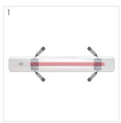
Mark locations of mounting brackets. Use a level tool if necessary. Then, remove brackets from GT1.0 Track.
