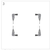
Drill holes for mounting screws with Ø4mm
