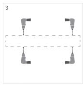
Drill holes for mounting screws with Ø4mm drill bit.
