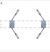
Secure brackets to the wall/table surface with the screws provided.
